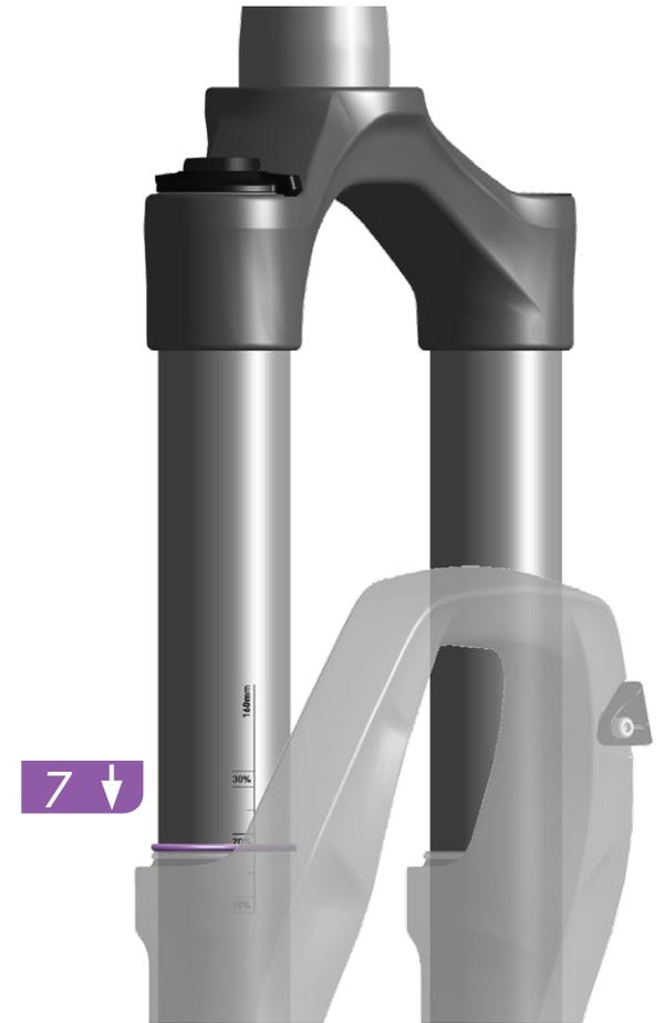
**Solo Air™ and DebonAir™ only:** Compress the fork through at least 50% of its travel five more times to equalize positive and negative air pressures.
