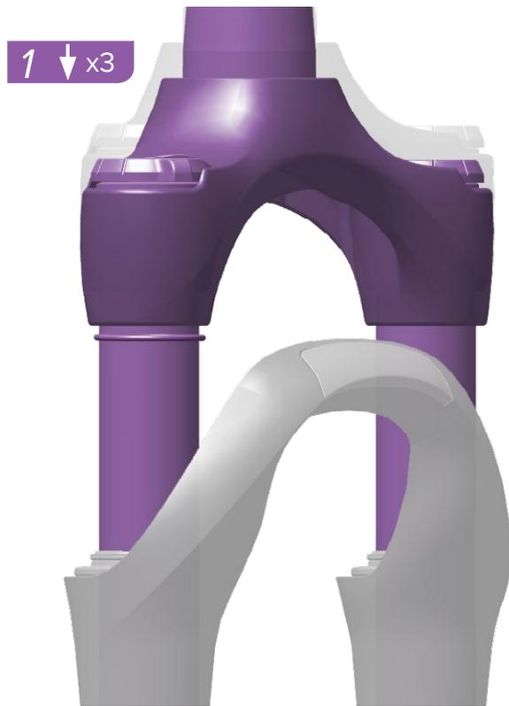
With riding gear on, and an assistant holding the bike, stand on the pedals, and compress the fork three times. Then sit or stand in your normal riding position.
