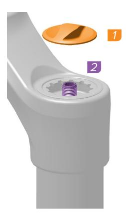
Pressurize the air spring to the recommended starting air pressure.
