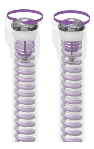
External spring **preload** adjustment compresses or decompresses the spring without initiating travel.
