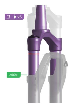
**Solo Air and DebonAir only:** Compress the fork through at least 50% of its travel five times to equalize positive and negative air pressures.
