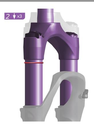
With riding gear on, and an assistant holding the bike, stand on the pedals, and compress the fork three times. Then sit or stand in your normal riding position.
