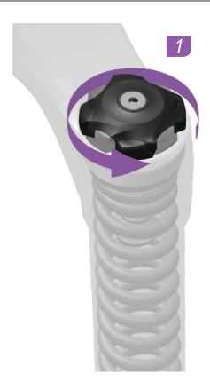
Turn the preload adjuster knob counterclockwise until it stops.
