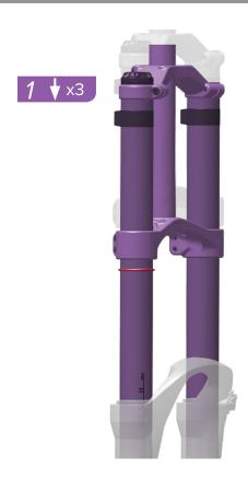
With riding gear on, and an assistant holding the bike, stand on the pedals, and compress the fork three times. Then sit or stand in your normal riding position.
