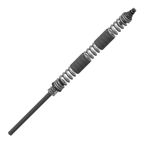
Spring preload adjustment can be used to fine tune sag, but preload does not change spring rate and is not a substitute for the proper coil spring weight.
