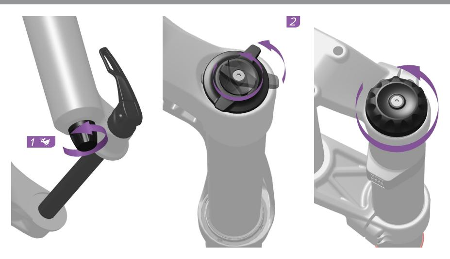
Before setting sag, set the dampers to the full open positions. Rotate the knobs counter-clockwise until they stop.
